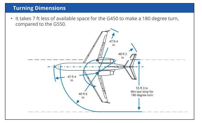
On the ground, that means the G450 can make 180 degree turn in a shorter, narrower taxi-way  $\dots$
