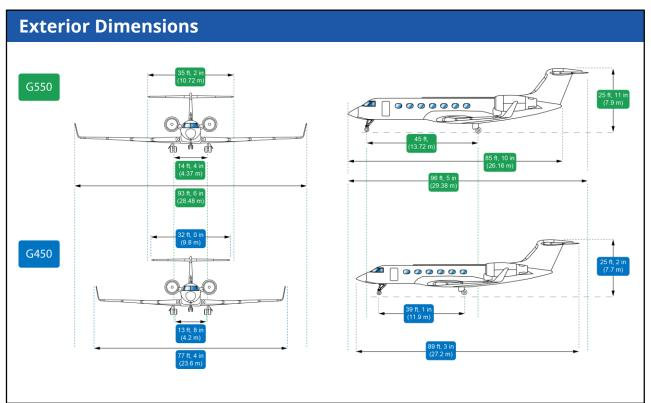
The G450 is about 10% shorter. Though the heights are similar. And the G450 has about 8% shorter wing and tail span.
